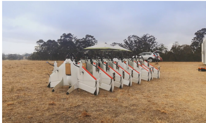
Figure 3: Google Wing reportedly experimented with using tailsitters for parcel delivery. The project was cancelled due to tailsitter instability.
