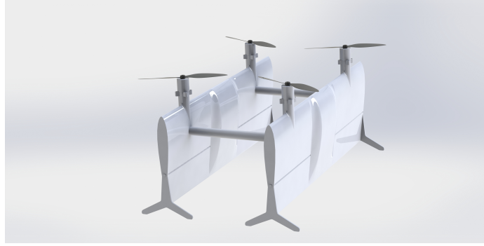
Figure 4: Concept rendering of final docked configuration.
