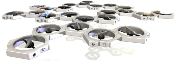
Figure 6: Distributed flight array developed at ETH Zurich by Oung et al.
